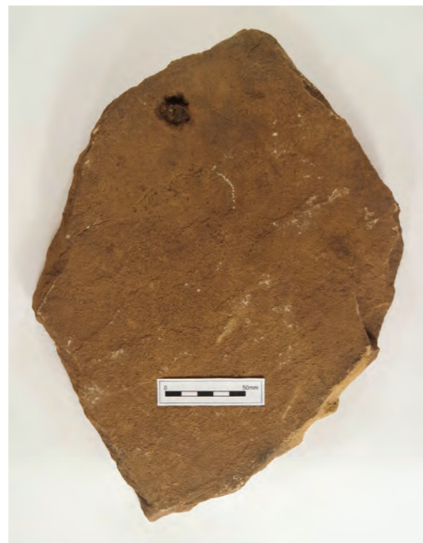
Fig 6.6 Complete stone roof tile with nail placed off-centre, from the roofing of building G106. © DoA
